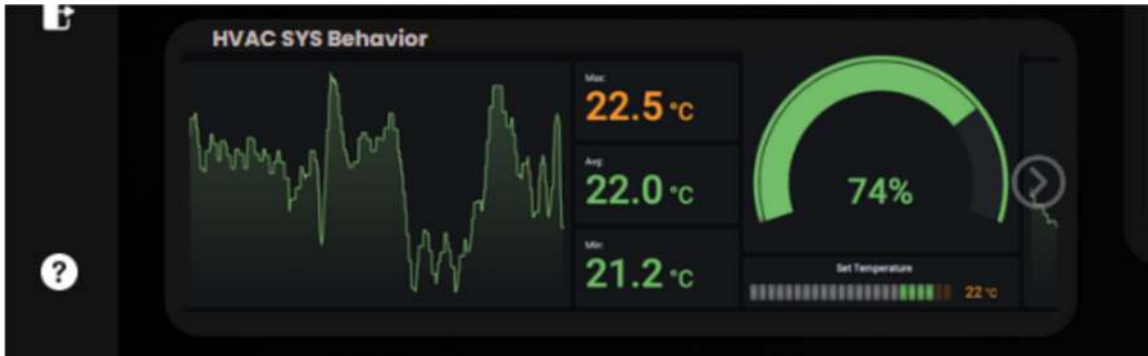
Figure 29 : Dashboard Comportement HVAC
